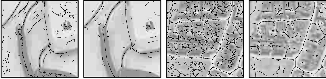
Figure 13: Examples of differential geometric ridge detection (without thresholding): (a)–(b) dark ridges from a detail from a telephone image at scale levels t = 16 and 64 , (c)–(d) bright ridges from an aerial image at scale levels t = 16 and 64 .
