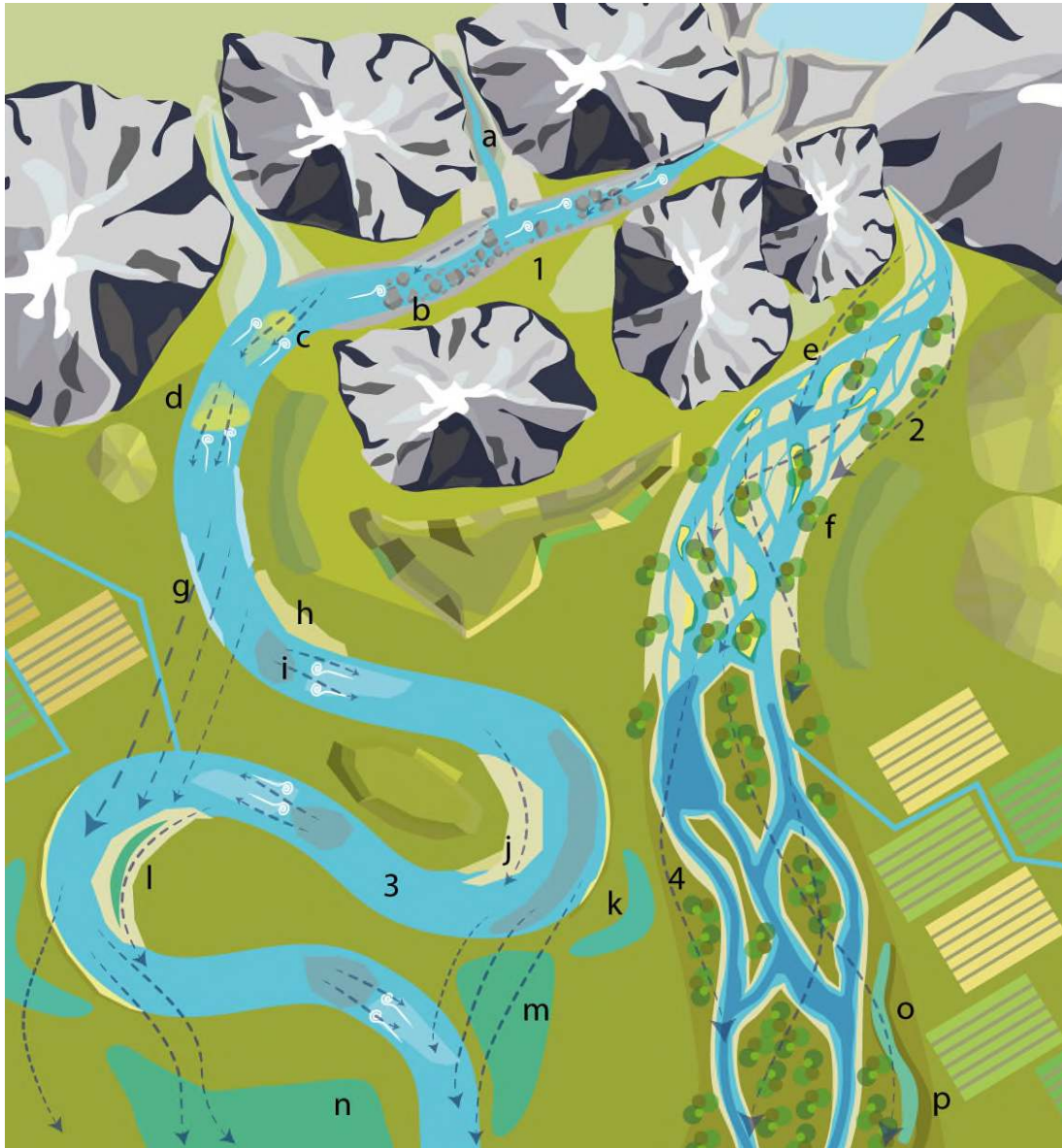
Figure 1: Illustration of catchment complexity: scales and features that influence hyporheic exchange flows. Spatial changes in surface topography, land use and vegetation, drive geomorphological and hydrological changes at valley and reach scale. At catchment scale, variations in surface topography shapes valleys and channel types. Feature 1 refers to confined valleys characterized by straight channels, meandered and braided, and the following floodplain features: scour holes and gravel splays (a). The straight channel presents in-channel cascades (b) geomorphic features. Feature 2 refers to braided channel morphology with multi-thread channel, an undulating floodplain of bars and islands. In-channel geomorphic units are several types of bars (e), such as mid and lateral bars, and vegetated islands (f). Feature 3 represents a sinuous-meandering floodplain with occasional oxbow lakes and backwater swamps (m, n, k) and in channel: longitudinal bar (c), transverse bar (d), counterpoint bar (h), pond-riffle (i), point bar (l), chute channel (j). Feature 4 indicates an anabranching valley with multi-thread channels including abandoned channels (o) and backwater swamps (p). The channel can be quite deep and include islands covered with vegetation. The symbol * refers to irrigation system of the adjacent agricultural fields.
