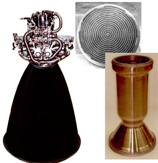
Figure 15. OME engine, injector, and combustion chamber hardware. 33
