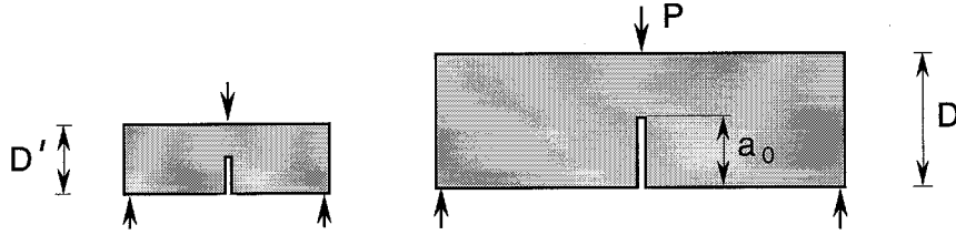
Figure 1. Geometrically similar structures of different sizes, with large similar cracks or notches.
