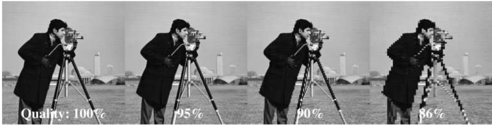
Fig. 1. Application of image blurring filter with varying degrees of output quality. Four levels of output quality are shown: 100%, 95%, 90%, and 86%.
