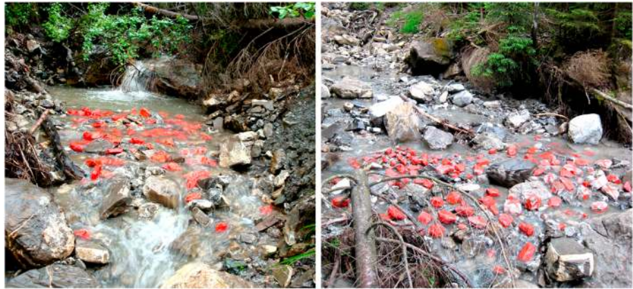
Figure 3. Tracer particles in the Erlenbach stream. (left) RFID campaign 2009, tracer insertion point I2. (right) RFID campaign 2010, tracer insertion point I4 (cf. Figure 1).
