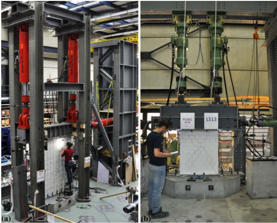
Fig. 6 a Photos of test stands for quasi-static cyclic wall tests on prototype walls (PUP1-5) and b Model walls (PUM1-5)
