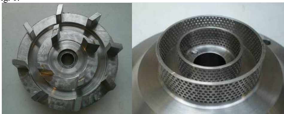
Fig. 1: Double rotor (left) and standard emulsor double screens (right) for the 150/250 MS Silverson
