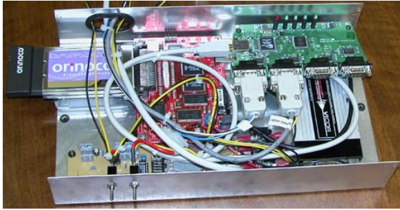
Figure 2: Some of the electronics onboard the helicopter: An Intel Stayton board with a 400Mhz XScale processor interfaces to the SICK LMS laser via a high speed RS422 serial link, and to all other devices (compass, GPS, IMU) via RS232. The communication to the ground is established via a 802.11b wireless link.
