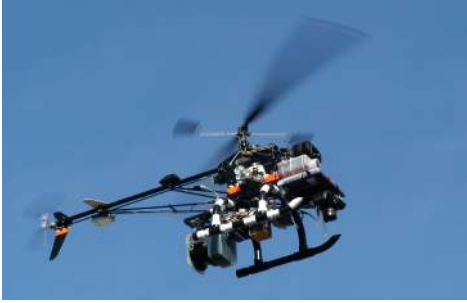
Figure 1: Instrumented helicopter platform: The system is based on the Bergen Industrial Twin, with a modified SICK LMS laser range finder, a Crossbow IMU, a Honeywell 3-D compass, a Garmin GPS, and a Nikon D100 digital camera. The system is equipped with onboard data collection and processing capabilities and a wireless digital link to the ground station.
