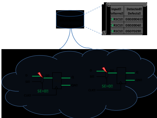
Fig. 6. Logic test intra-cell defect grading
