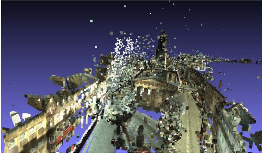
Figure 6: Noise, in this case snow, must be removed before surface creation.
