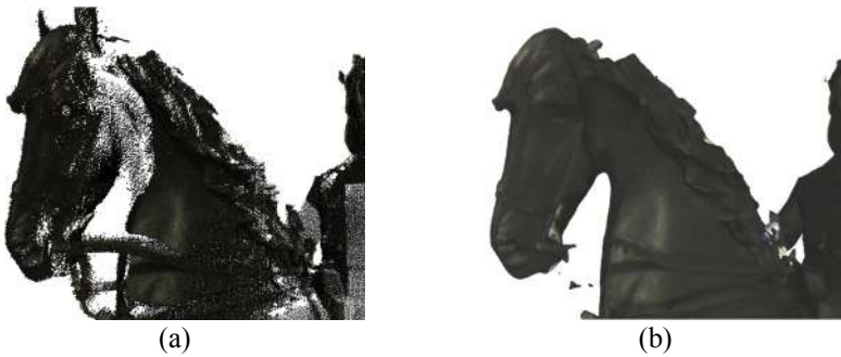
Figure 5: Point cloud and solid mesh representation. (a) High detailed point cloud, dissolves on approach. (b) Lower detailed solid mesh, retains solidity but loses definition.
