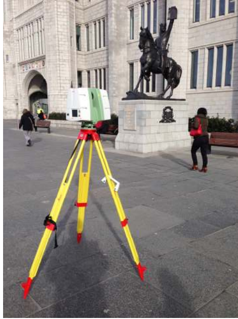
Figure 2: Scanning statue (Leica C10 scanner).
