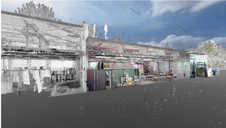
FIG 7: Point Cloud 2 from laser scan of the use case, as generated by company 1
