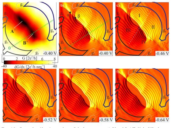
**Figure 4.** Set of images taken with varying gate voltage applied to the upper top gate  $g_4$  (solid purple line). The black solid line draws the biased gate with a fixed voltage throughout the whole set, the thin gray line belongs to grounded gates. (a) Conductance map with  $V_g = -0.4$  V. (b)–(f) Numerical derivatives with respect to *x*-direction. The black dashed lines gives a guide to the eye to follow the separation of the inner fringes.
