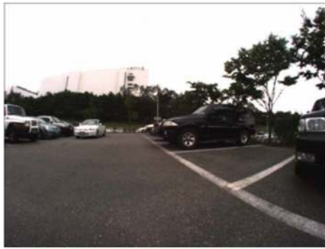
Fig. 32. One of two failed situations. As the laser beam direction was almost perpendicular to the normal direction of the parked vehicle's front, the corresponding range data could not be acquired.
