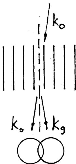
Fig. 2. A plane incident wave, vector k_0 , inclined to the optic axis (dashed line) produces a diffracted beam k_g by interaction with "Bragg planes" or any periodicity in the projected specimen lattice potential. A wide enough convergent beam will produce overlapping discs, whose relative phase can be determined from the overlap region.
