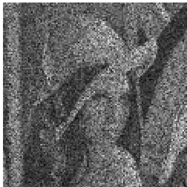
Figure 4.6: An 8-bit grayscale image with normal distributed gain and offset nonuniformity, standard deviations 0.3 and 25 respectively.
