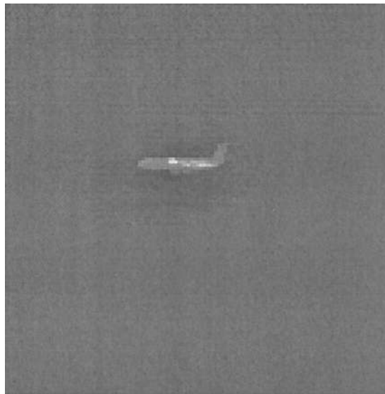
Fig. 14. Frame of Fig. 13 corrected by use of 500 consecutive frames per block and correlation factors \alpha_6 = \beta_6 = 0.95 .
