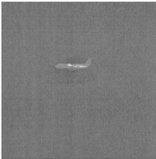
Fig. 15. Frame of Fig. 13 corrected by use of 800 consecutive frames per block and correlation factors \alpha_6 = \beta_6 = 0.8 .
