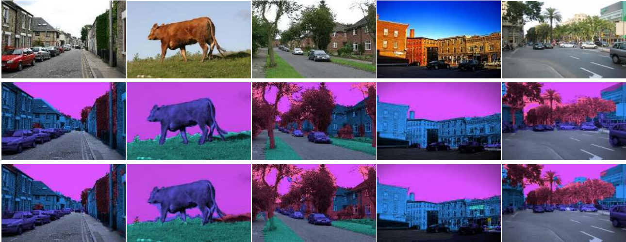
Figure 4: The results of scene labeling on the Stanford Background dataset. First row: input image; Second row: ground-truth; Third row: predicted image. Colors on images indicate labels — identical colors on ground-truth and predicted images indicate a correct labeling
