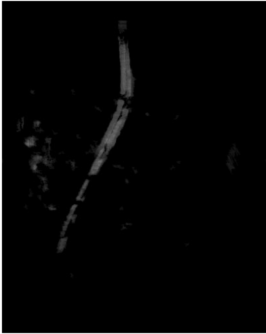
Figure 4: Figure where each individual pixel stores the number of times a foreground object was detected at that pixel. Note how the road is clearly distinguished from other areas due to objects moving on the road.
