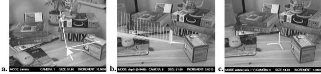
Figure 5. Insertion of the virtual frame into a desk scene: a) initial placement into one of the reference images by specifying the desired location of the frame’s origin; b) the frame’s trajectory along the epipolar line in another image; c) subsequent orientation adjustment.
