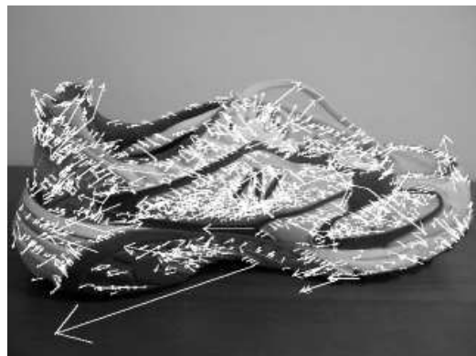
Figure 2. SIFT keypoints extracted from a 640 \times 480 image of a sneaker. The algorithm found 1533 features shown as white arrows, with size and direction corresponding to feature scale and orientation, respectively.
