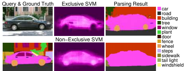
Figure 4. Exclusive vs. non-exclusive SVM output. The exclusive SVM has a very low response for areas of the car that have attached objects, like the wheels. This would penalize candidate object masks that include the wheel pixels. By contrast, the non-exclusive SVM has a high response for all parts of the car, and the resulting pixel labeling favors classes with larger area, which typically correspond to background or occluded classes.
