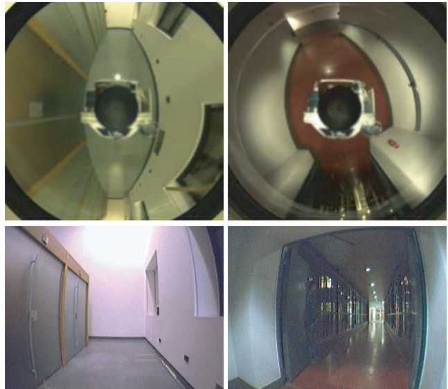
Figure 1. Examples of omnidirectional images (top) and standard images (bottom) taken at the same position. These examples illustrate that omnidirectional vision is more powerful for recovering the whole spatial layout of the scene from a single image.
