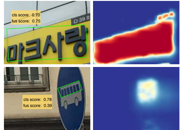
Figure 1: Visualization of detection results and semantic segmentation feature maps. Left: The detection result with classification score and fusion score. The fused score is calculated by Re-Score mechanism. Right: The feature map for text segmentation.
