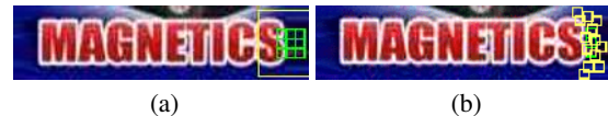
Figure 3: Illustration of our deformable convolution. (a) normal convolution; (b) deformable convolution with 3 \times 1 convolution. The green boxes indicate convolutional kernels. The yellow boxes mean the regions covered by receptive fields. The receptive fields out of the image are clipped.
