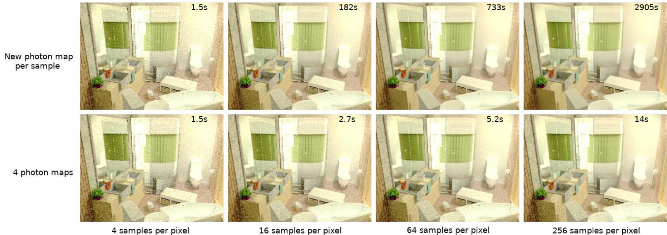
Figure 6. Trade off between rendering time and quality. Each photon map contains approximately 3M stored photons.
