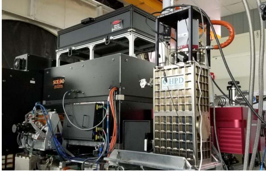
Figure 4. Photo of the SCExAO instrument, with the NIR cameras at the three outputs: from left to right, SAPHIRA, MEC and CHARIS.
