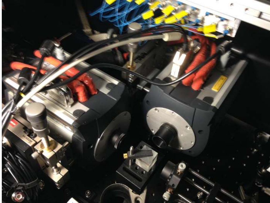
Figure 5. New design of VAMPIRES using two EMCCD cameras.
