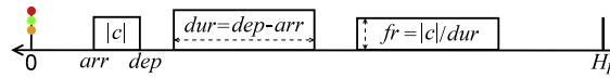
Fig. 2. Example of clusters on a route, each can be defined by three of the five attributes.
