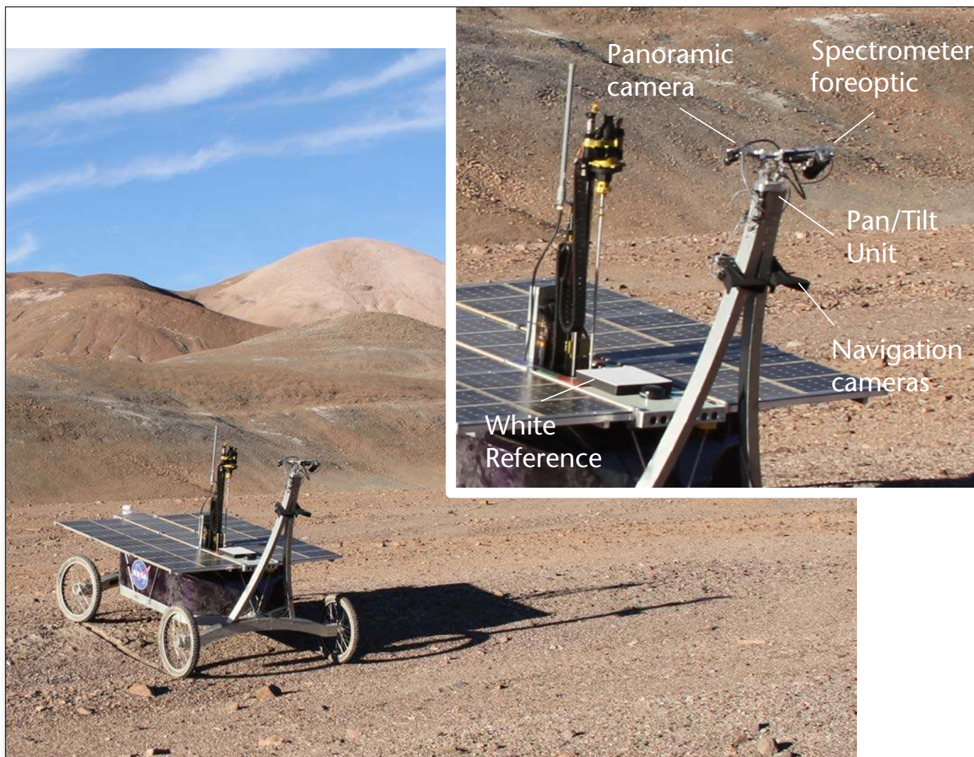
Figure 5. The Main Components of Zoë's Vis-NIR Spectrometer System.
