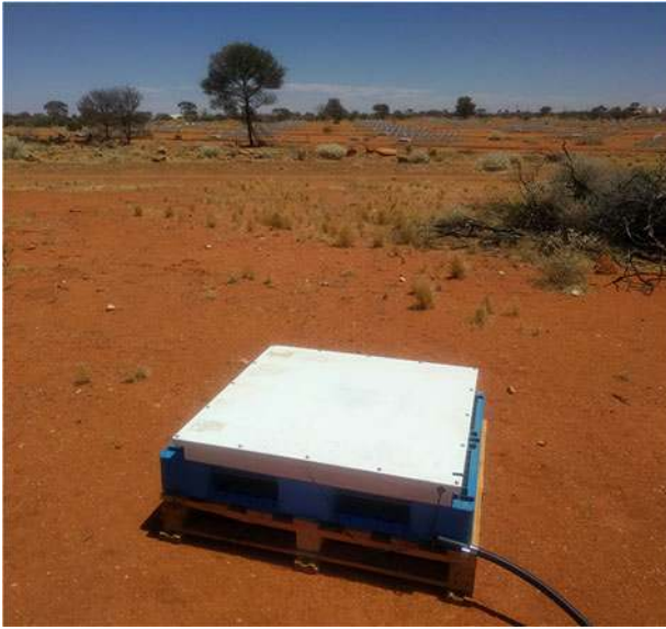
Figure 9. The prototype SKAPA cosmic ray detector (white box) deployed near the MWA core at the MRO. It is raised off the ground with pallettes to avoid surface water. Power and data return are enclosed via the black cable housing. The detector has been tested to ensure compliance with MRO RFI requirements and has been detecting cosmic ray muons since its deployment in October 2018. Photo credit: Justin Bray.
