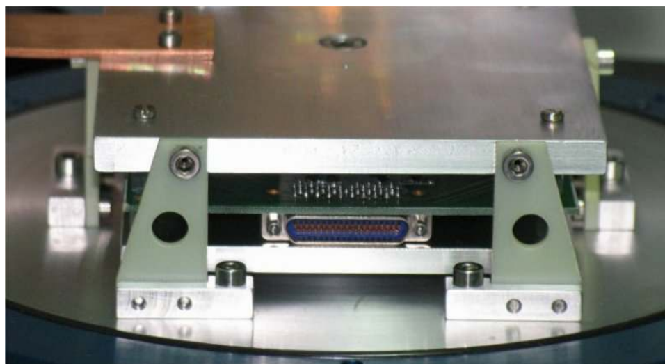
Figure 7. The detector head PCB is shown sandwiched between the baseplate and a CCD clamping plate. A 37-way Glenair connector carrying all CCD signals is also visible at the centre.
