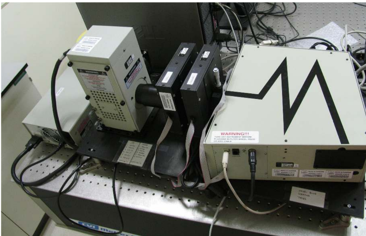
Figure 1. From left to right: stabilized lamp power supply, light source, filters wheels and monochromator.
