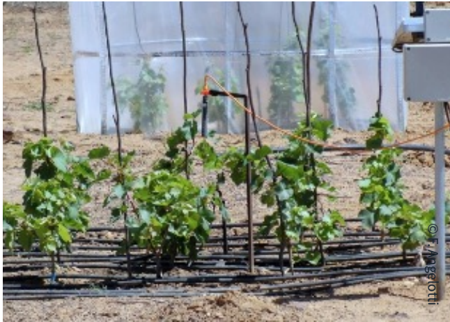
Open top chambers for studying the impacts of increased air CO 2 concentration in Petrolina, Brazil
