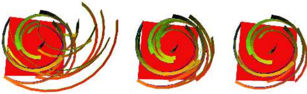
Figure 7. Streak bands in a vortex flow computed on a full grid and sparse grids of level 0 (left), 1 (middle), and 4 (right).
