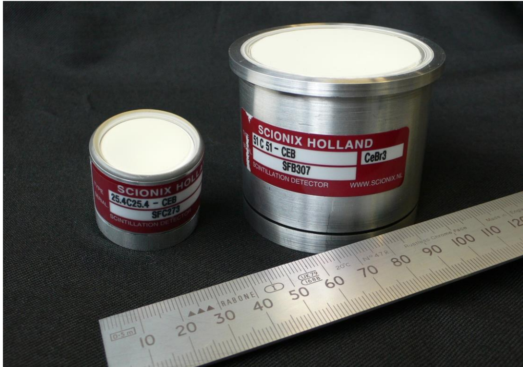
Fig. 1 – Picture of two of the \text{CeBr}_3 encapsulated samples used in this study, left 1"×1" sample SFC 273 (proton irradiated) and right 2"×2" sample SBF 307.
