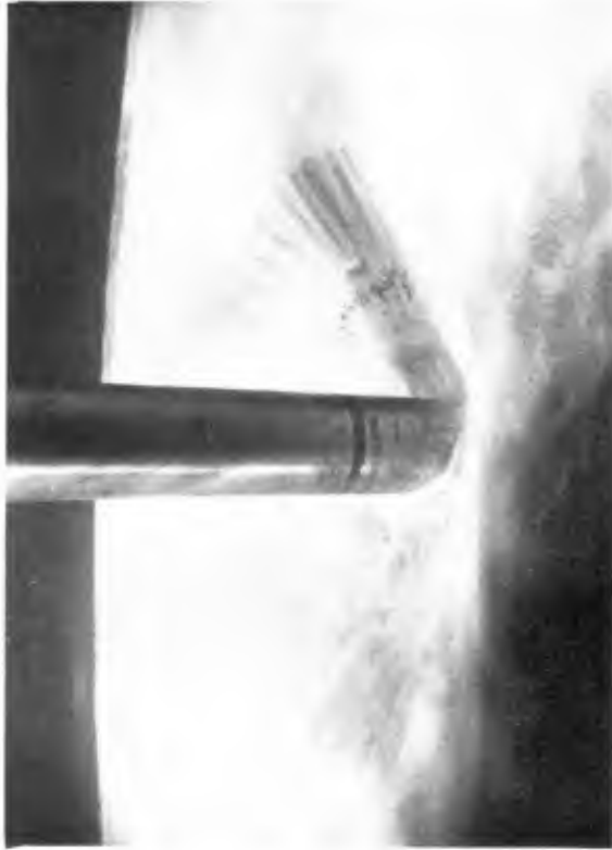
FIGURE 4a Photograph of sand scour depression around 50mm cylinder at maximum u_* .
