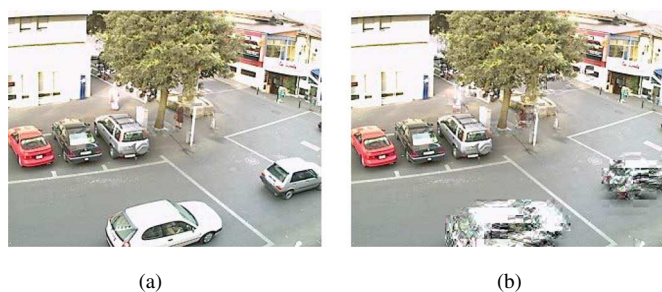
Fig. 11. Privacy protection scrambling in a real video surveillance setting: (a) original sequence and (b) with transform-domain scrambling.
