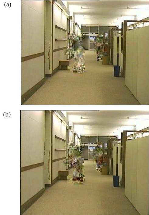
Fig. 4. Transform-domain scrambling for Hall Monitor : (a) 63 ac coefficients and (b) dc + 63 ac coefficients.
