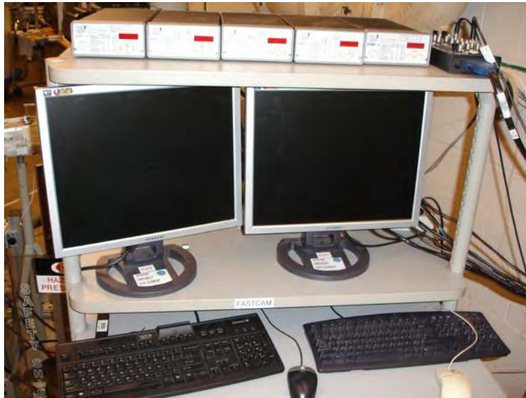
Figure F.14: Endeveco Model 136 DC amplifiers, hydraulic control computer, and shadowgraph control computer
