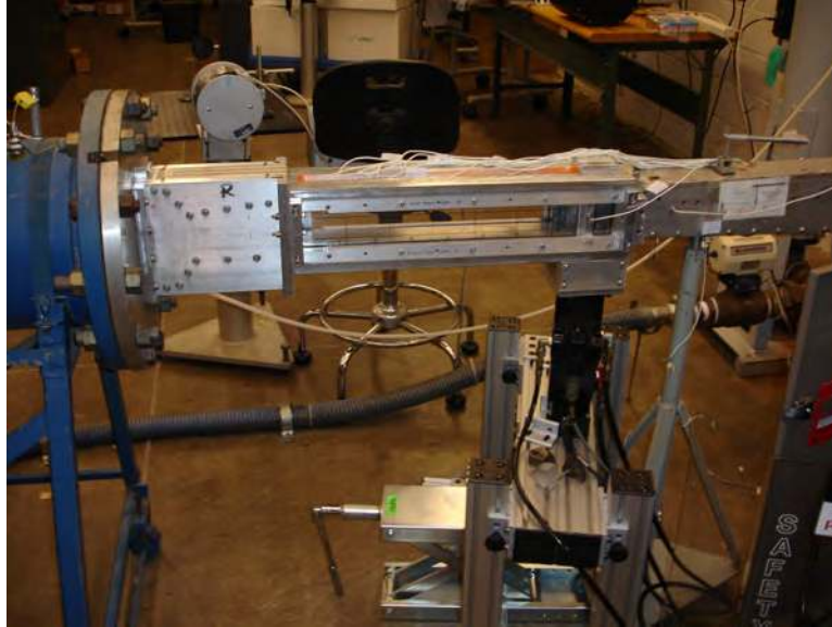
Figure F.12: Nozzle, test section, and hydraulic actuator
