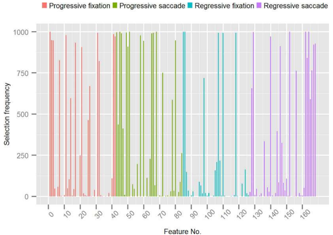
Fig 4. Frequency of features selected during training of the best performing classification model grouped by progressive/regressive fixation- and saccade features. The Y-axis shows the number of times a feature in the original feature set was selected by the recursive feature elimination algorithm (SVM-RFE) during the 10 x 100 cross-validation with internal feature selection. The X-axis shows the features (represented by their index in the dataset) grouped by progressive/regressive fixation- and saccade features.
