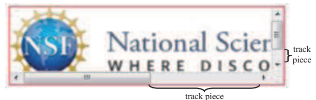
Figure 4. Placing an image which exceeds the width and height of the div in a div container will result in the appearance of the horizontal and vertical scrollbars. The increment and decrement track pieces of the two scrollbars will also occur. The increment track pieces are visible by default.
