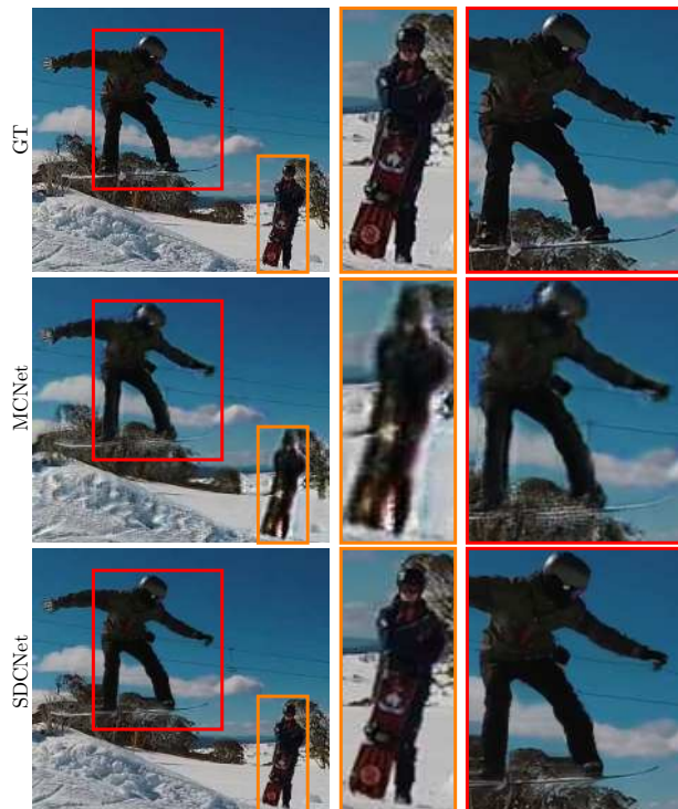
Fig. 6. Comparison of frame prediction methods. Shown from top to bottom are Ground-truth image, MCNet and SDC-Net results. SDCNet is shown to provide crisp and sharp frames, with motion mostly in good alignment with the ground-truth frame. MCNet results on the other hand appear blurry, with artifacts surrounding the persons (framed in red and orange). MCNet results also show checkerboard artifacts near the skis and on the snow background.
