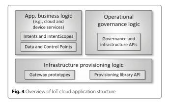
logic components (e.g., cloud services and device services); resource provisioning and deployment logic (custom or stock component provisioning); and operational governance logic.
