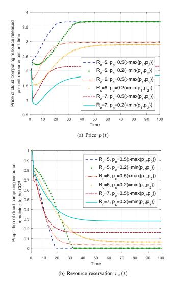
Fig. 6. Dynamic computing resource pricing and allocation in the ECC system versus different  $R_c$  and  $p_c$ .
