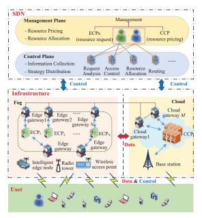
Fig. 1. Architecture of SDN-based resource pricing, sharing and user scheduling in an ECC system.
