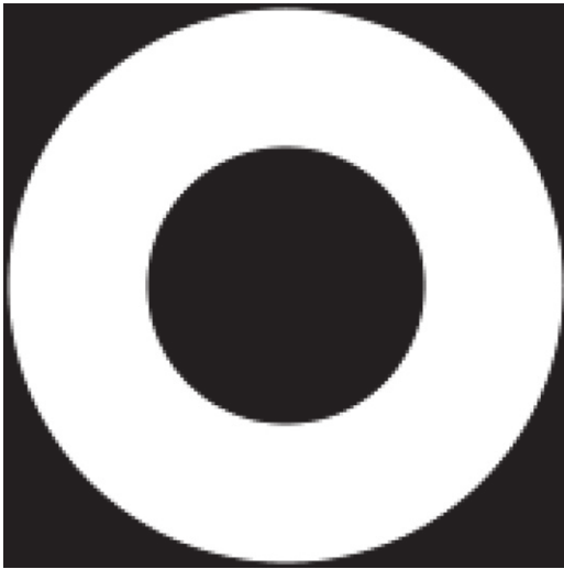
Figure 1. The convolution kernel used in modeling the effect of a focus offset on the PSF.
