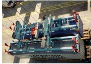
(b) QC with a double lifting trolley (Source: Jordan, 2002)
