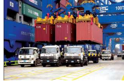
(c) QC with a triple lifting trolley (Source: China Communications construction company, 2010)
