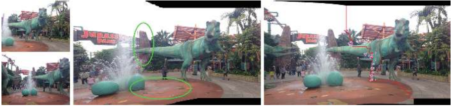
Fig. 1. Comparison of global alignment and our seam-guided local alignment. Left: Input images. Middle: Stitching result by APAP [25] (all features are used). Right: Stitching result by our method (only features around the final stitching seam are used).
