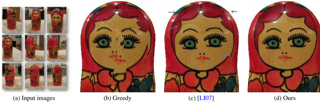
Figure 1: Overview of our contribution. (a) The input photographs. (b) Back-projecting the photographs onto the geometry of the doll by selecting the best image for each triangle in a greedy manner results in strong artifacts. (c) Optimizing the selection of images for texture coherence according to [LI07] alleviates the problem, but seams and broken texture are still noticeable. (d) Our texture montage results are nearly seamless.
