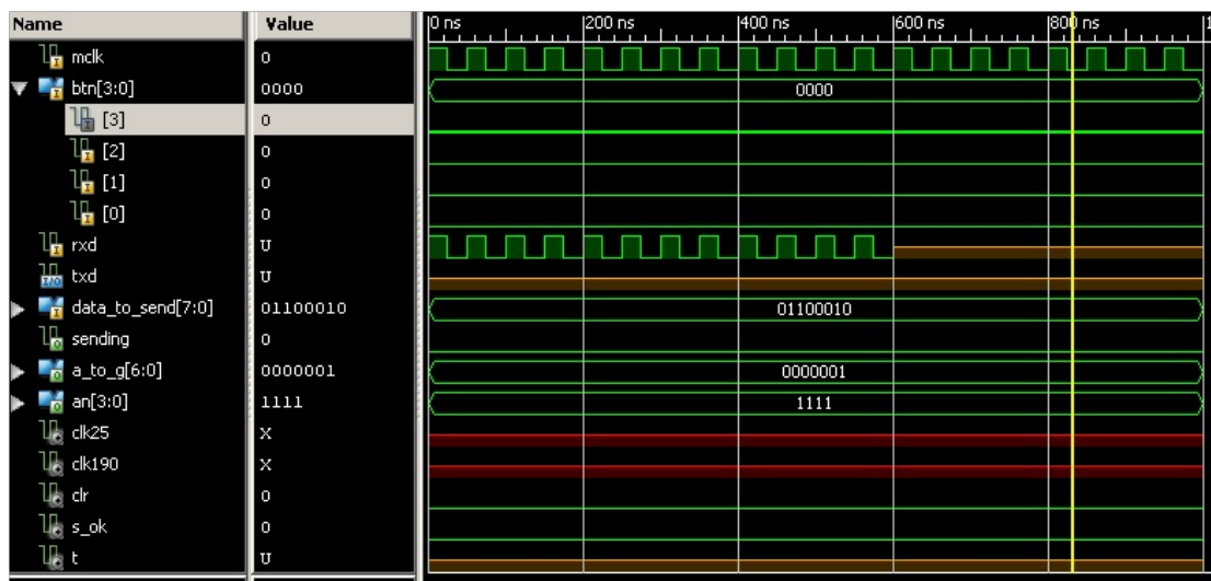
Figure 6 RTL VHDL simulation snapshot of the UART design.
