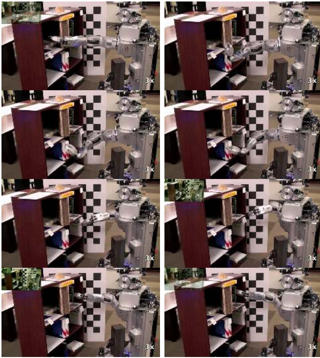
Fig. 5: Snapshots of the robot planning to a goal position in a cluttered environment.
