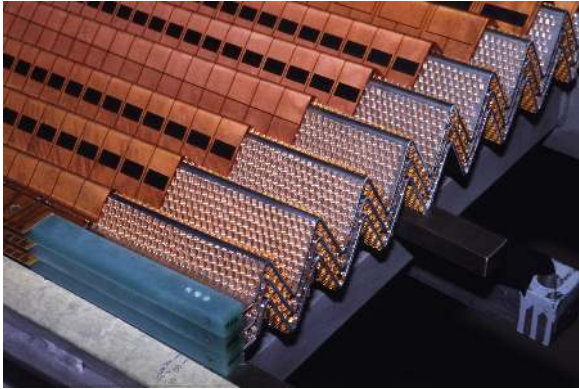
(a) LAr calorimeter accordion structure, Particles enter from the bottom left of the picture. The copper electrodes are spaced from the lead by honeycomb.
