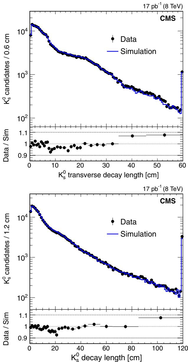
FIG. 4 (color online). Transverse decay length (left) and decay length (right) distributions of the  $K_S^0$  candidates in data and simulation. The ratio histograms are shown with neighboring bins merged until the relative statistical uncertainty falls below 2%. The last bin contains all candidates that are above the plotted range.
