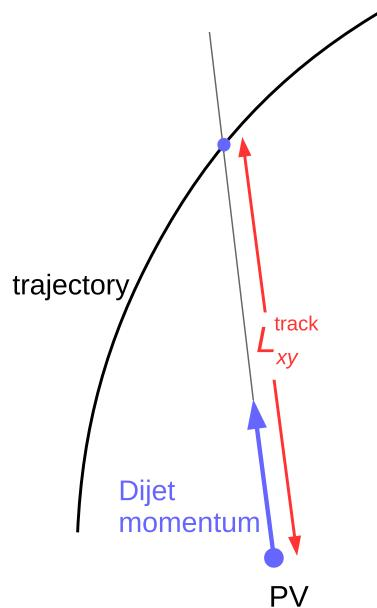
FIG. 1 (color online). Diagram showing the calculation of the distance  $L_{xy}^{\text{track}}$ . In the transverse plane,  $L_{xy}^{\text{track}}$  is the distance along the dijet momentum vector from the primary vertex (PV) to the point at which the track trajectory is crossed.
