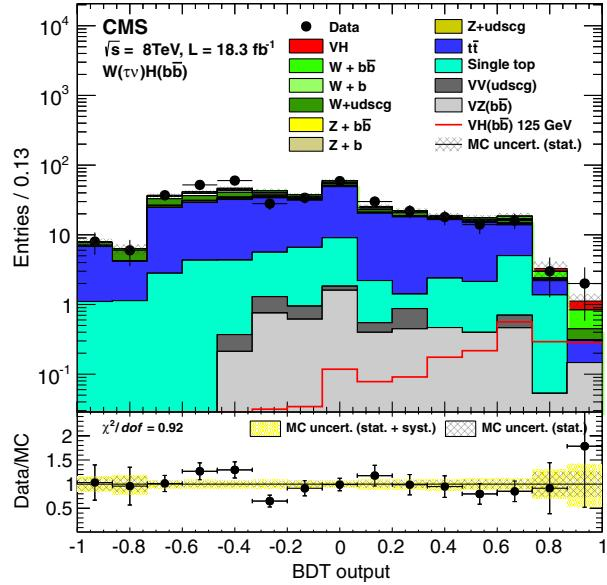
FIG. 12 (color online). Postfit BDT output distributions for  $W(\tau\nu)H$  for 8 TeV data (points with error bars), all backgrounds, and signal, after all selection criteria have been applied. The bottom inset shows the ratio of the number of events observed in data to that of the Monte Carlo prediction for signal and backgrounds.
