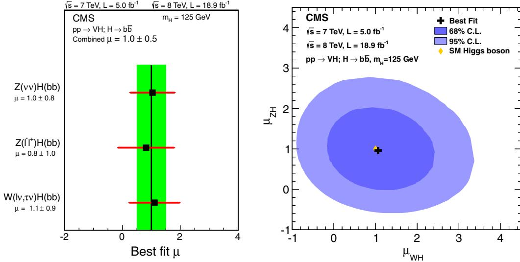
FIG. 7 (color online). Left: best-fit value of the production cross section for a 125 GeV Higgs boson relative to the standard model cross section, i.e., signal strength  $\mu$ , for partial combinations of channels and for all channels combined (band). Right: best-fit values and the 68% and 95% C.L. contour regions for the  $\mu_{ZH}$ ,  $\mu_{WH}$  signal strength parameters for a 125 GeV Higgs boson.
