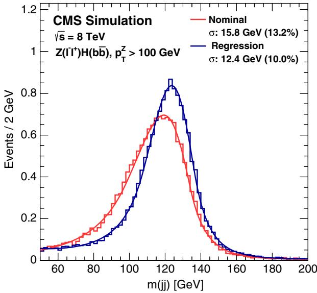
FIG. 1 (color online). Dijet invariant mass distribution for simulated samples of  $Z(\ell\ell)H(bb)$  events ( $m_H = 125$  GeV), before (red) and after (blue) the energy correction from the regression procedure is applied. A Bukin function [66] is fit to the distribution and the fitted width of the core of the distribution is displayed in the figure.
